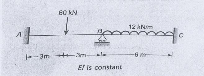
Q.8) Analyse the given beam shown in the figure using slope deflection method.
