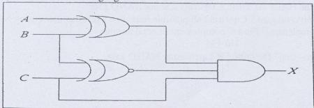
What is the required input condition (A,B,C)to make the output X=1, for the above logic circuit?
